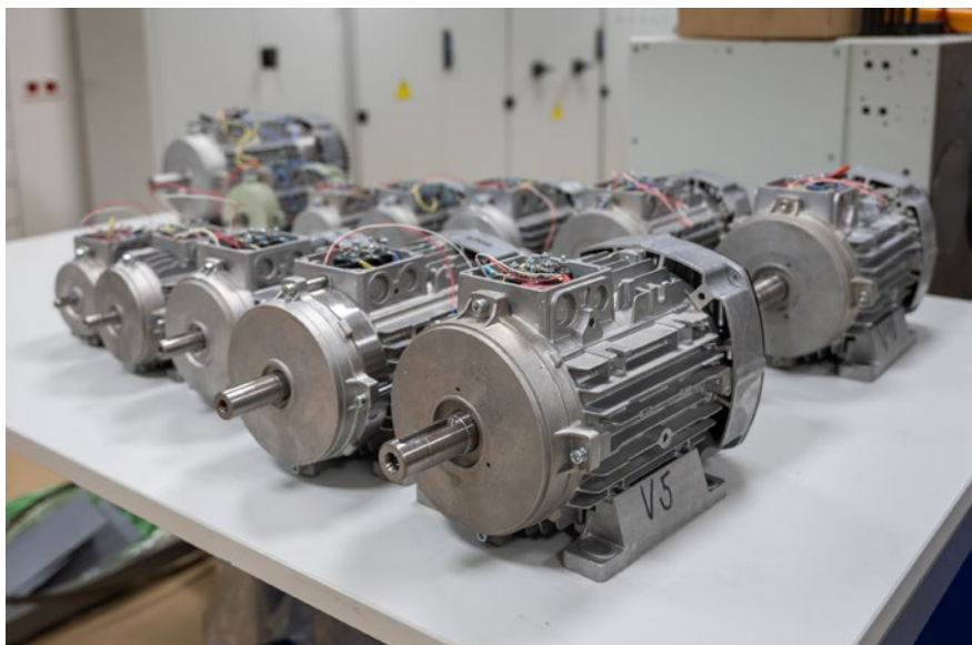
Unique single-phase motors from the FEEC with permanent magnets.
