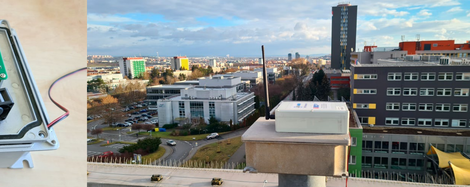
LoRaWAN Sniffer device developed by the project, on the top of the T12 building roof, monitoring LoRaWAN networks in Brno.
