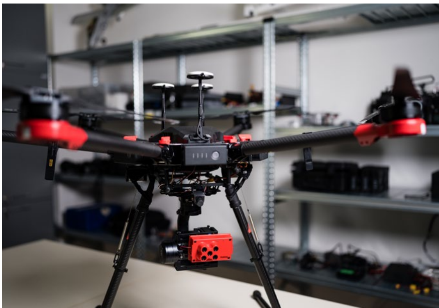
A big drone is equipped by multispectral camera with five lenses.
