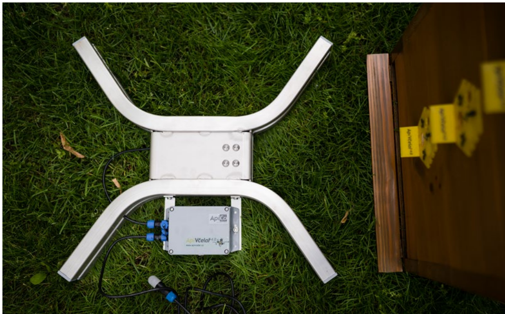
A scale is one of the main parts of smart beekeeping. According to a graph a beekeeper can recognize what is happening inside the bee hive and if bees bring nectar there.
