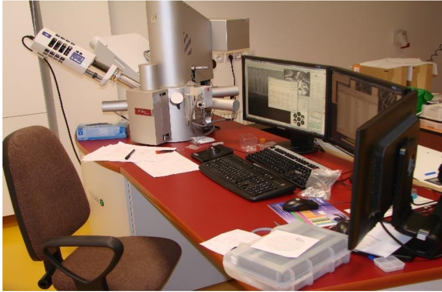
REM TESCAN microscope in the department laboratory
