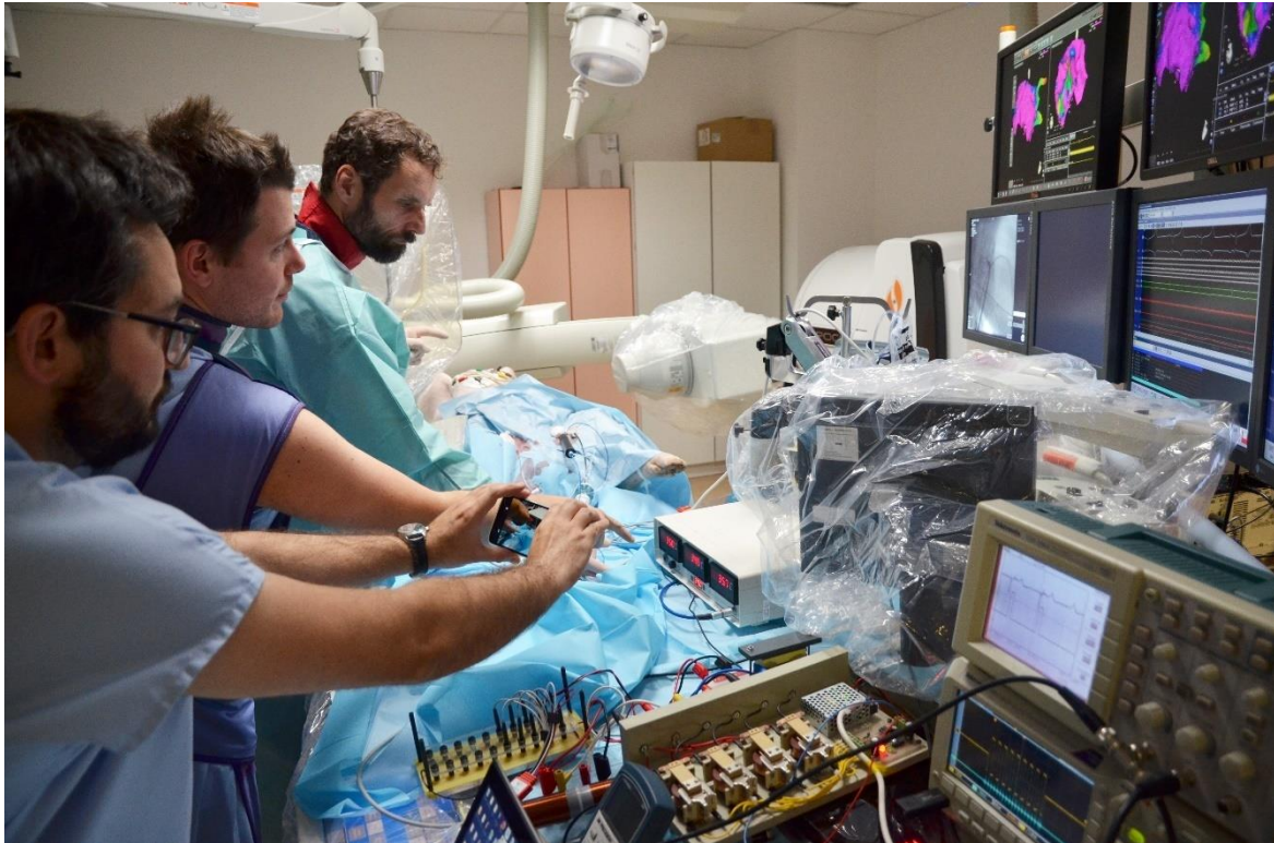
Testing of electroperforational UVEE device for cardio arrhythmia removal
