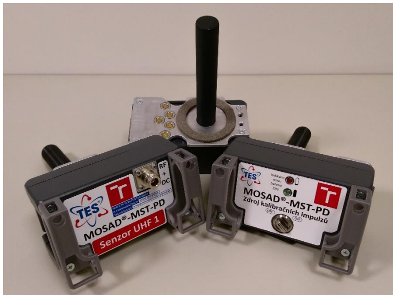
Partial discharge UHF signal sensor and calibration impulses source
