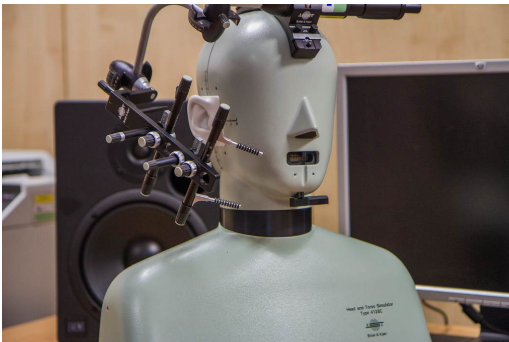
Head and torso simulator with artificial ear and mouth for measurement of electroacoustic characteristics of telecommunication devices such as communicators, microphones and mobile phones
