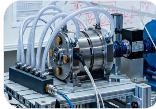
Slitted rotor Induction machine 12 kW at 50 000 rpm
