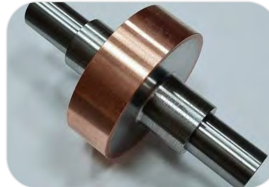
Coated rotor test sample for verification of surface speed up to 300 m/s
