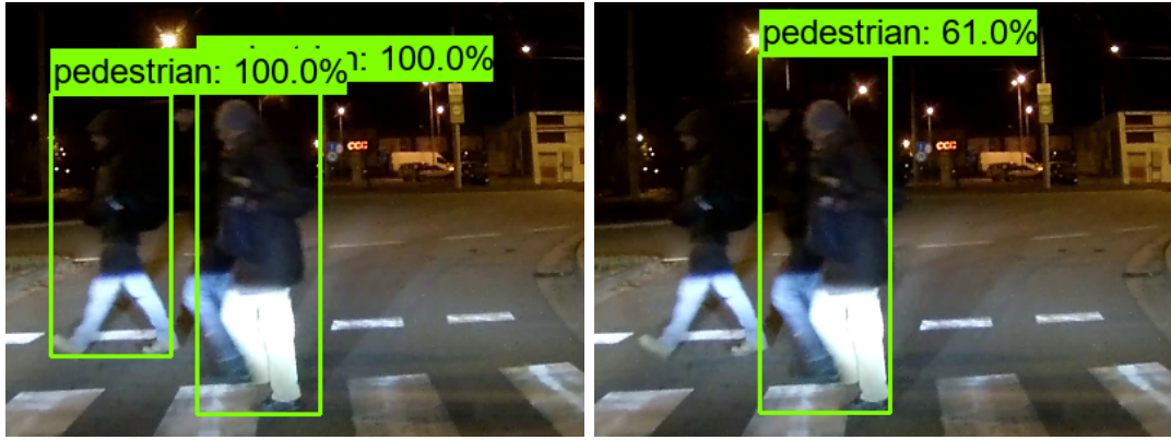
Figure 2: Examples of pedestrian detections by FRCNN Zemcik and SSD Zemcik respectively
