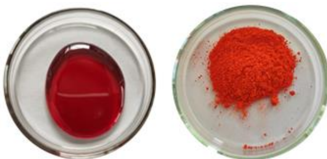
Image 3: IVS sample containing a ratio of S:DIB 70:30 wt. %.
