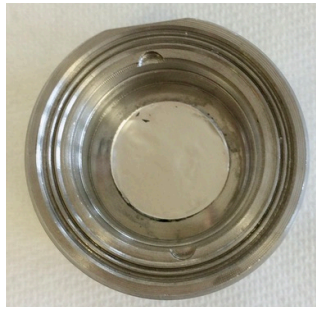
Figure 1: Complete Li/GPE/NMC cell
