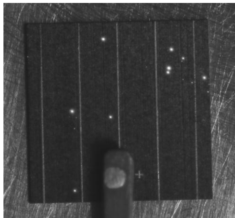
Figure 2: Light emission of defects on reversed bias solar cell, bias voltage U_r = 6.5 V, exposition time t = 10 s, temperature T = 297 K
