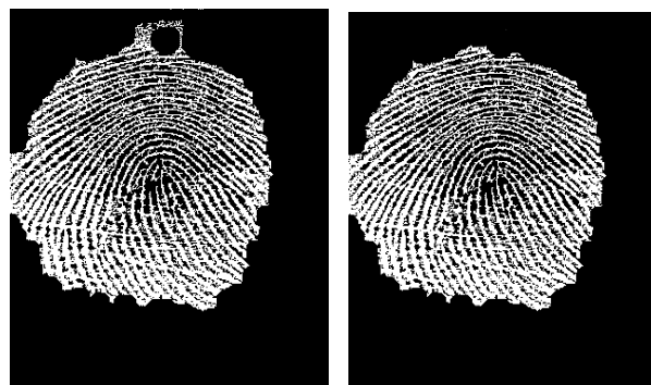
Figure 5: Segmentation before (left) and after (right) correction
