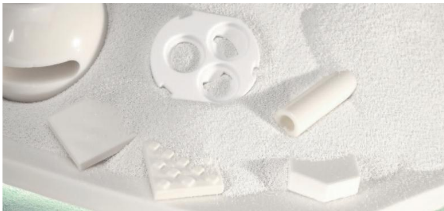
Figure 1: Corundum powder and sintered parts [1]
