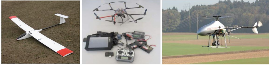
Figure 2: Three different UAV platforms: plane [1], multirotor [2] and helicopter [3].
