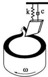
Picture 1. Model of regenerative chatter Picture 2. Geometry of turning
