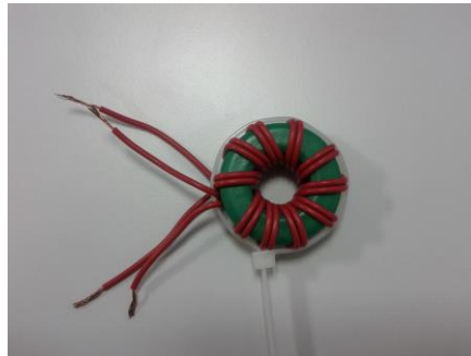
Figure 3 - The 1:1 transformer, windings together
