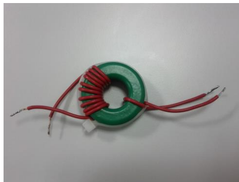
Figure 5 - The 10:1 transformer, windings on other sides
