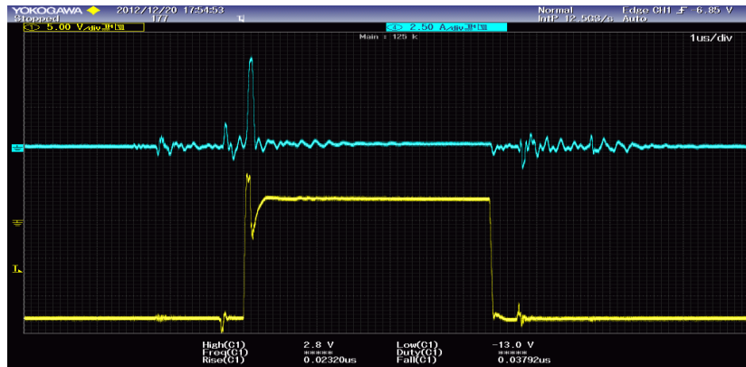
Figure 7 Proposed gate driver waveforms of GS voltage (yellow) and S current (blue), DC bus voltage 540V
