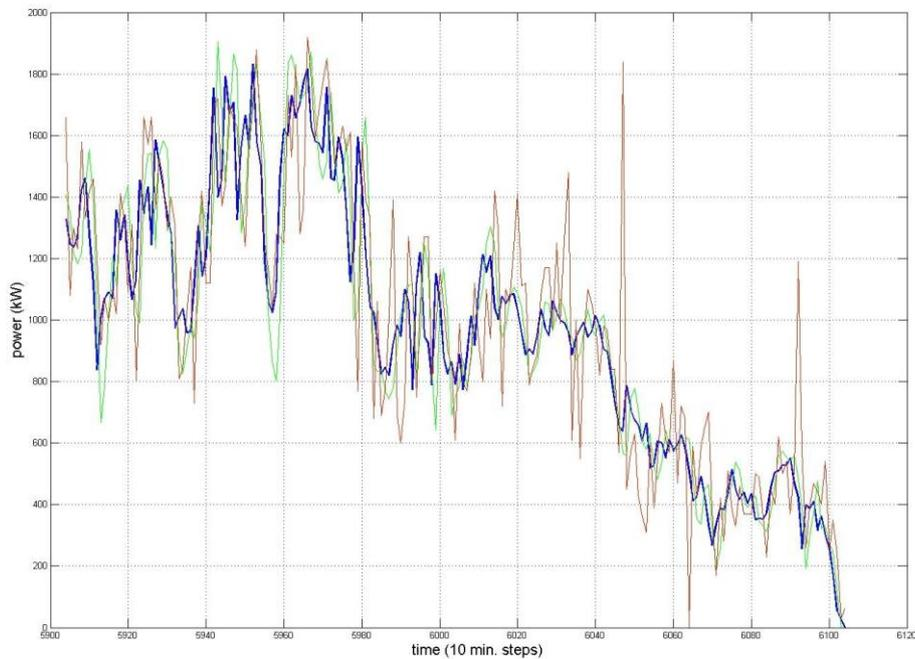
**Figure 1:** Prediction model sample (measured data are given by blue line, green line represents autoregressive model, red line represents Markov chain model).
