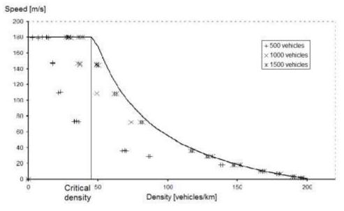
Figure 4: A relation between traffic speed and density in evaluating experiment
