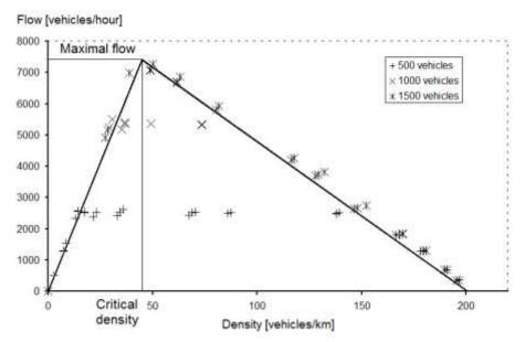
Figure 3: A relation between traffic flow rate and density in evaluating experiment
