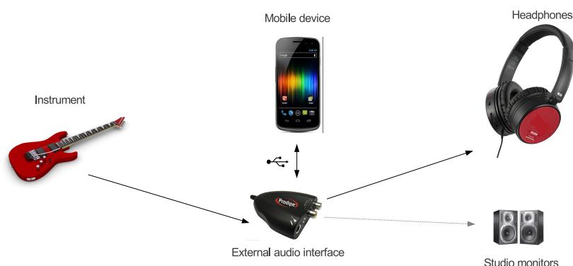
Figure 1: Hardware components and their connections
