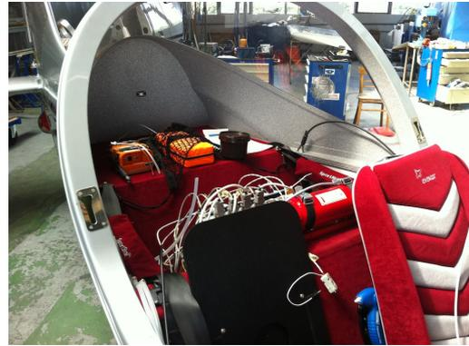
(b) Data acquisition system installation.
