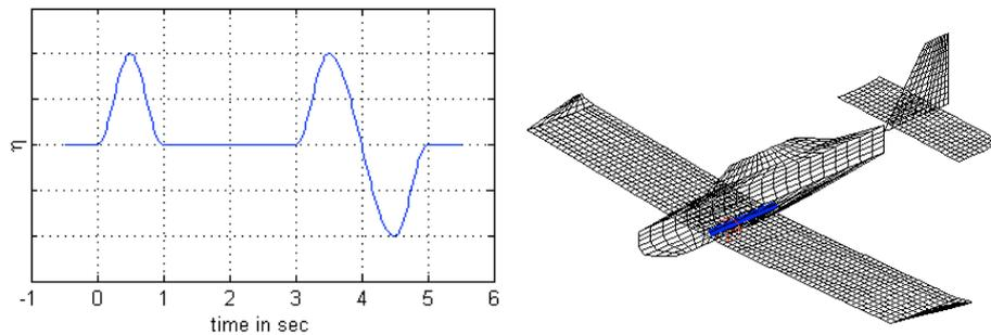
(a) The shape of elevator maneuvers used for identification – pulse (left), doublet (right). (b) Visualization of the model of the Sportstar RTC in Tornado.
