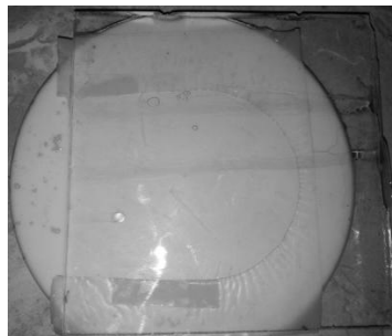
Figure 7: Teflon and glass with a Teflon foil with the possibility of air leak.
