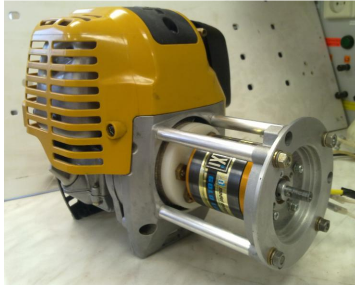
Figure 2 Electric generator and combustion engine connection
