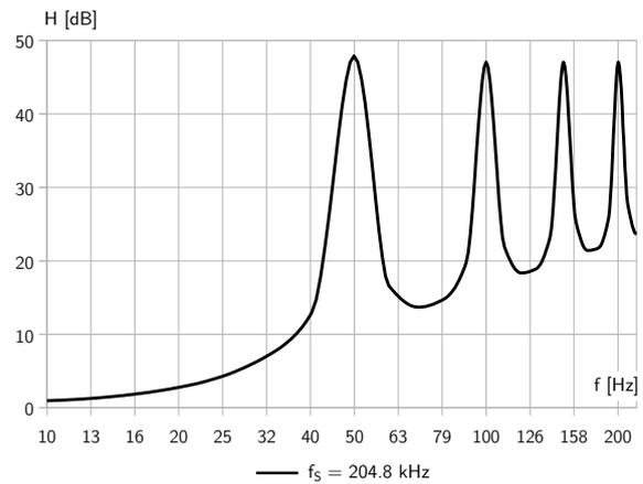
**Figure 7:** Series Mode Rejection Ratio
