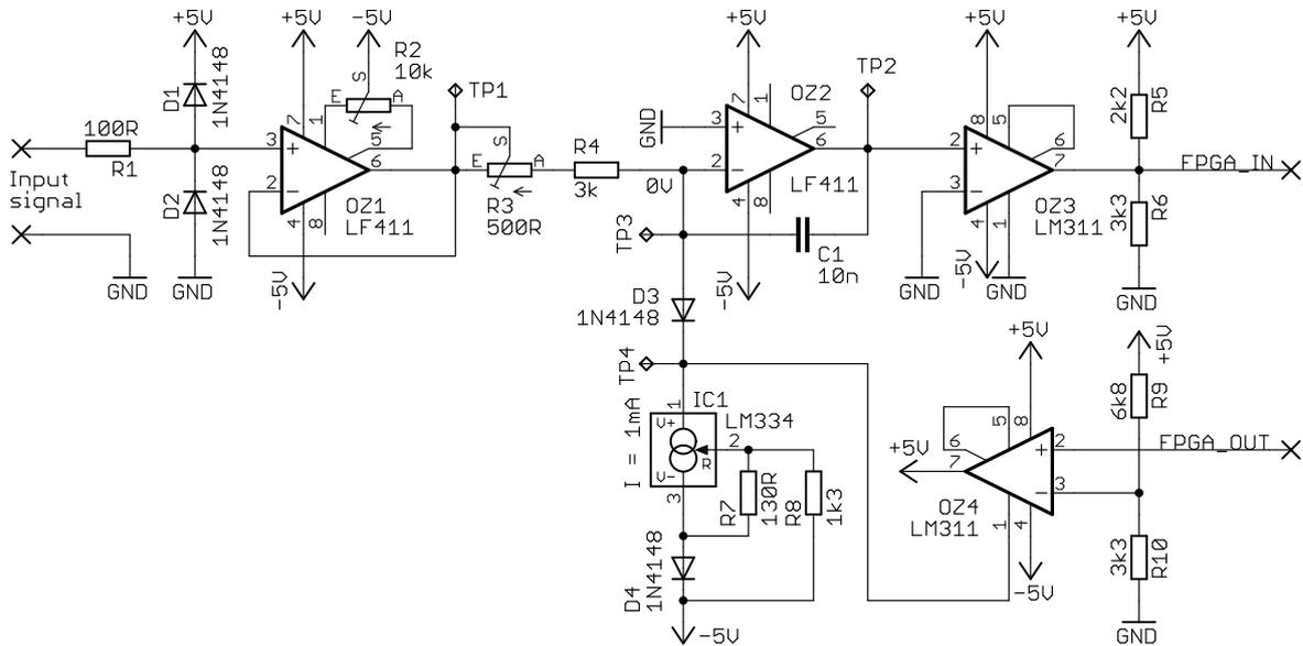
**Figure 4:** Schematic of Analog Circuitry
