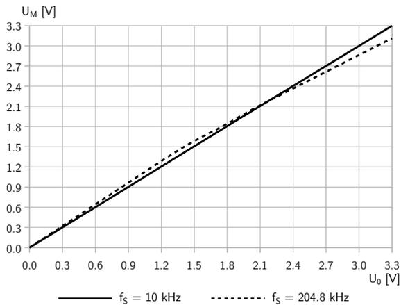
**Figure 6:** Transfer Function of ADC
