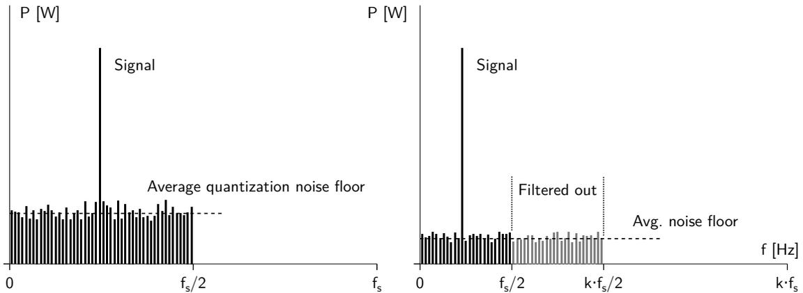
**Figure 2:** Quantization Noise
