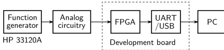
**Figure 5:** Block Diagram of Measurement Configuration
