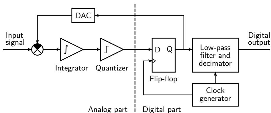
**Figure 1:** Block Diagram of Delta-Sigma ADC
