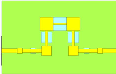
**Figure 2:** Layout of fractal low-pass filter with EBG
