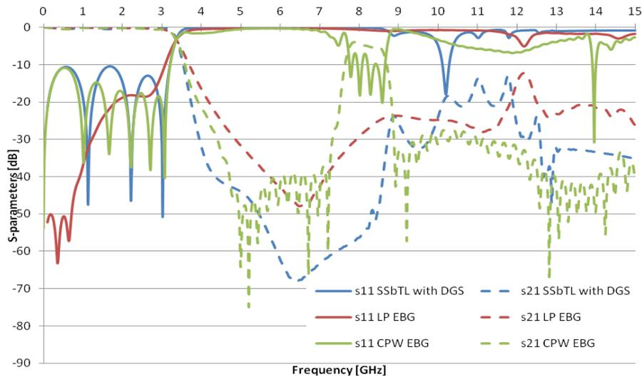
**Figure 4:** Frequency response of return loss  $S_{11}$  and insertion loss  $S_{21}$  of low-pass filter with reduced fractal DGS (blue line), low-pass filter with EBD (red line) and fractal CPW EBG low-pass filter (green line). Computed by CST
