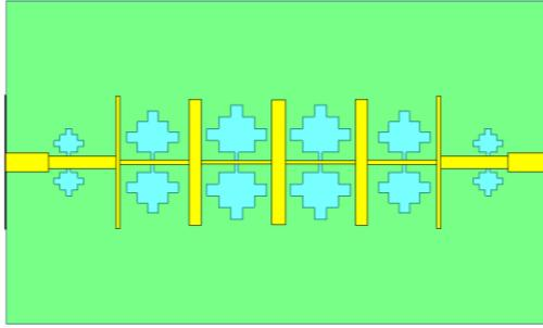
**Figure 1:** Layout of low-pass filter with reduced fractal DGS
