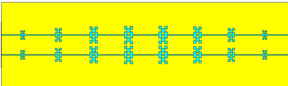
**Figure 3:** Layout of fractal CPW EBG low-pass filter
