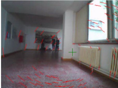
Figure 3: Optical flow caused by rotation of the vehicle.
