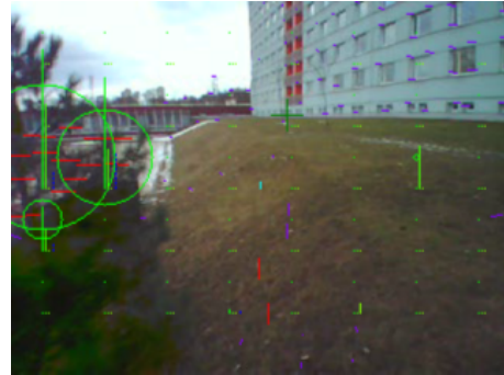
Figure 4: A tree detected when flying near by. The group of red lines indicates vectors above threshold.
