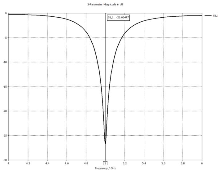
**FIGURE 4:** Frequency response of the return loss of the patch antenna.
