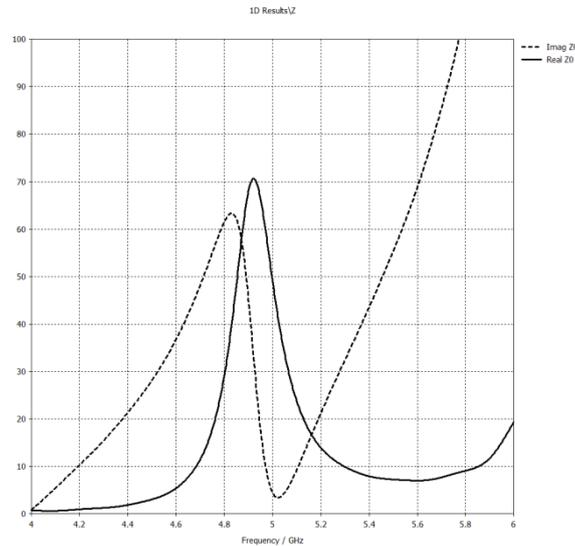
**FIGURE 5:** Input impedance of patch antenna.
