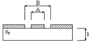
**FIGURE 2:** CPW feed structure.
