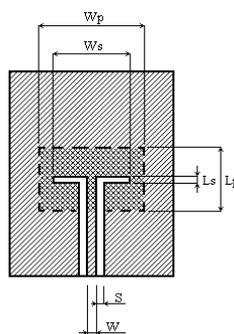
**FIGURE 1:** Basic configuration of patch antenna.
