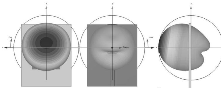
**FIGURE 6:** Radiation pattern of the patch antenna ( $G = 7.7$  dB @ 5 GHz).
