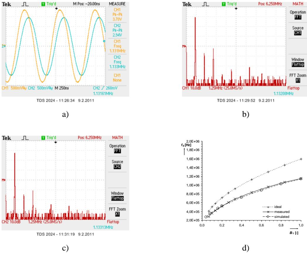
**Figure 3:** a) measured output responses, b) c) spectrum of both responses, d) dependence of oscillation frequency on current transfer  $B_1$ .
