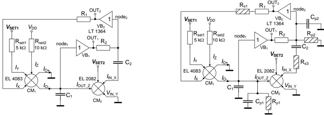
**Figure 1:** a) oscillator circuit, b) important parasitic influences in structure
