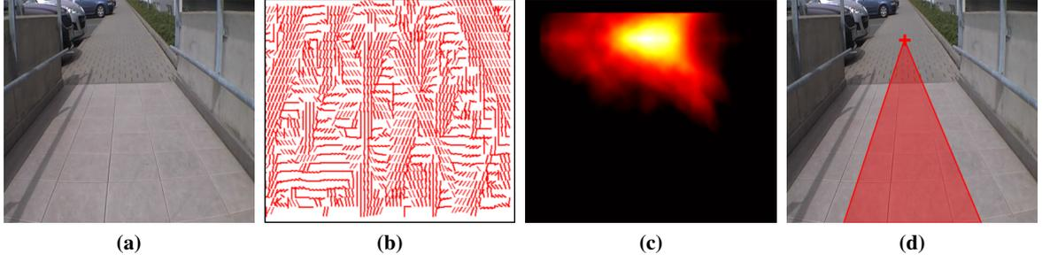
**Figure 1:** Input image (a), estimated dominant orientations (b), voting function (c), output (d).
