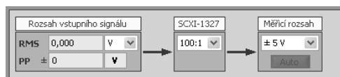
Figure 8: The software conception of user environment of measuring chain configuration of the module NI SCXI-1327.
