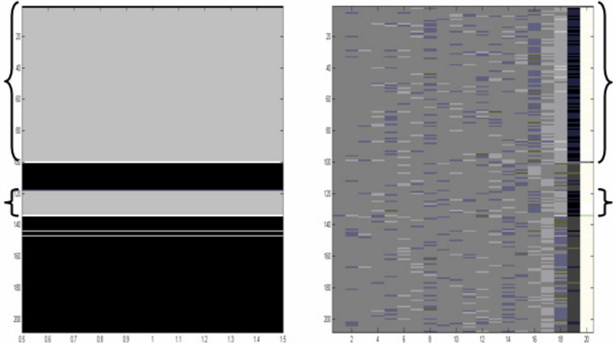
Figure 2: ECG record 102,60 000 samples, left side marks from MIT archive and vectors of parameters on the right side, normal rhythm and paced beats
