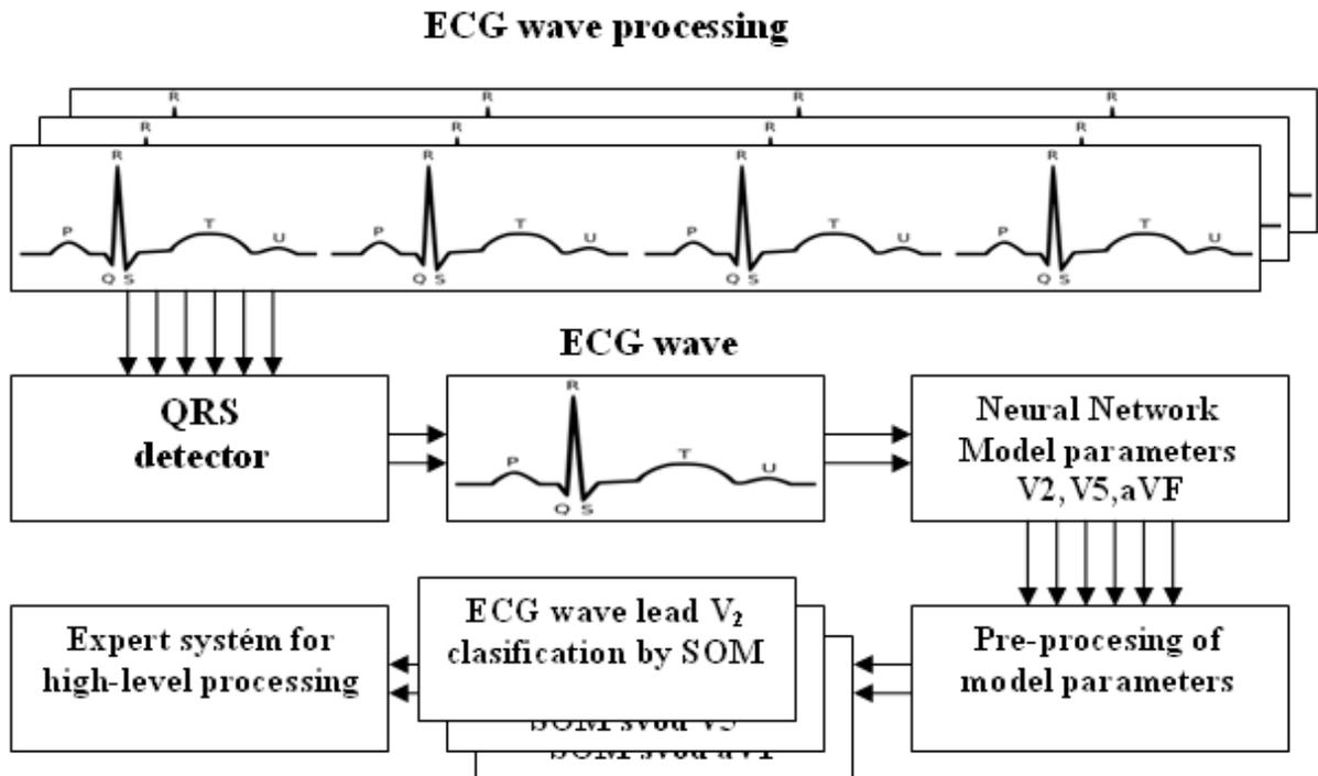
Figure 1: Process of ECG wave processing
