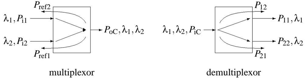
Figure 1: Two channel WDMX and WDDX.
