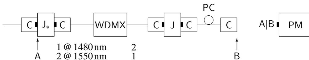
Figure 6: Measuring chain for directivity.
