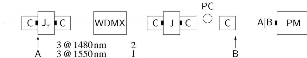
Figure 5: Measuring chain for isolation.
