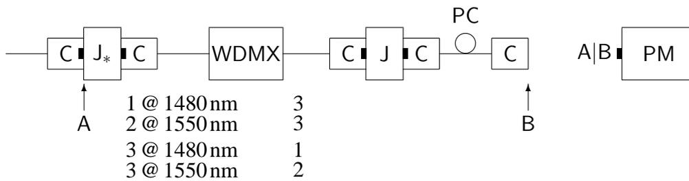
Figure 4: Measuring chain for insertion loss.
