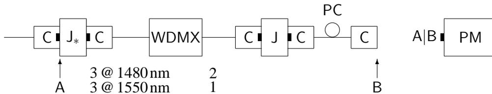
Figure 5: Measuring chain for isolation.
