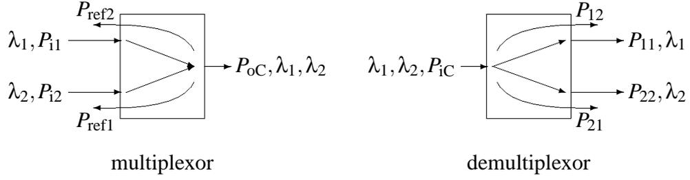
Figure 1: Two channel WDMX and WDDX.
