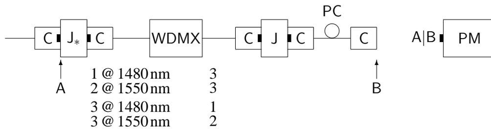
Figure 4: Measuring chain for insertion loss.
