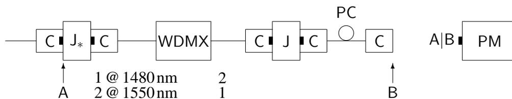
Figure 6: Measuring chain for directivity.
