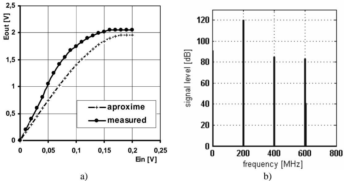
**Fig. 2:** a) *Transfer characteristic of amplifier* b) *Frequency spectrum of output signal*
