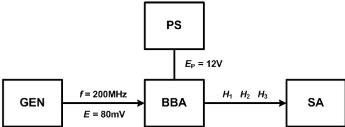
**Fig. 1:** Block diagram of measuring site
