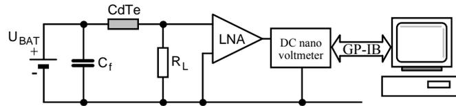
**Fig. 1:** Block diagram of the experimental set-up
