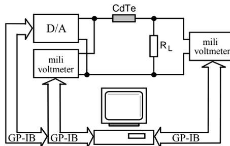
**Fig. 2:** VA characteristic measuring set up
