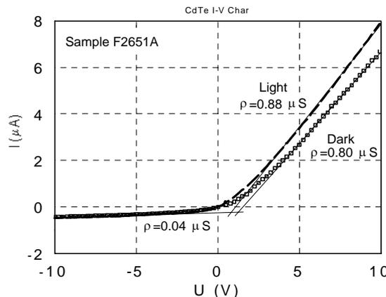
**Fig. 3:** VA characteristic in the dark and at the room temperature for sample 1
