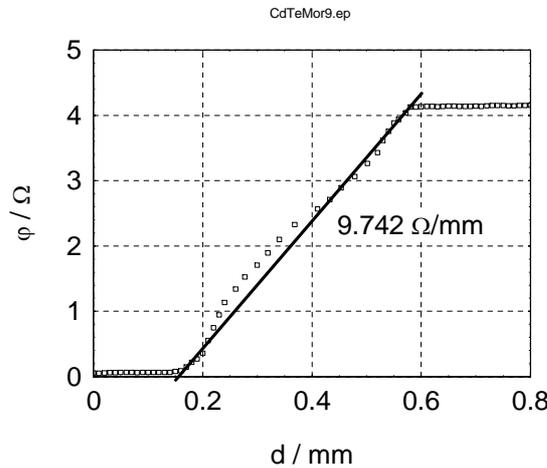
**Fig. 4:** Contact resistance was measured by DisPot and result for sample 1
