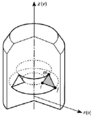
**Fig. 1:** *Element of axisymmetric solid*
