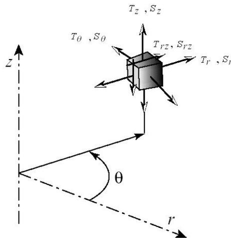
**Fig. 2:** *Axisymmetric strain and stresses*
