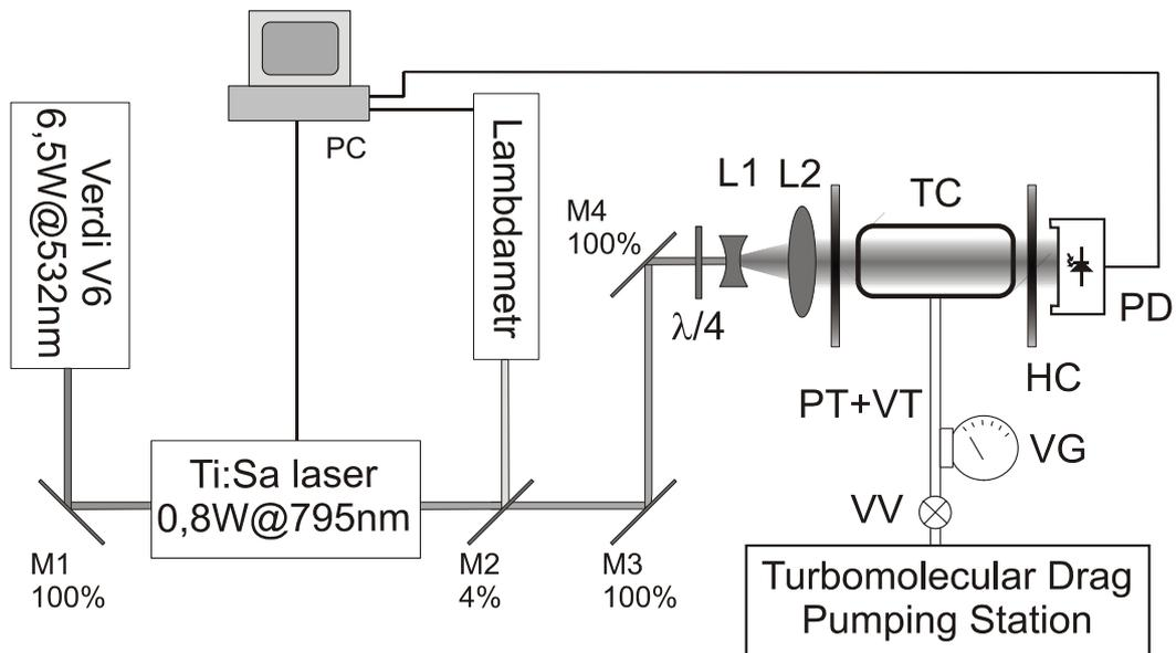
**Fig. 1:** *Experimental set-up for optical pumping of rubidium. M1, M2, M3, M4 - mirrors,  $\lambda/4$  - quarter-wave retardation plate, L1 - diverging lens, L2 - converging lens, TC - target cell, HC - Helmholtz coils, PD - photodetector, PT - plastic tube, VT - vacuum hose and VV - vacuum valve*
