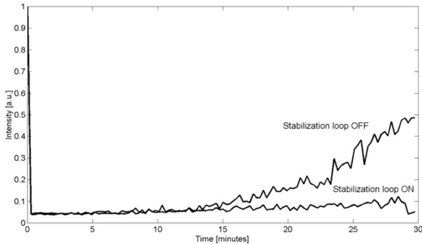
**Fig. 3:** *Illustration of the effect of using the stabilization loop*
