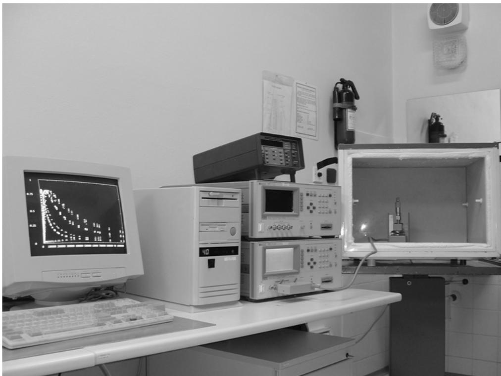
**Fig. 1:** *Equipment for the measurements in the frequency domain*
