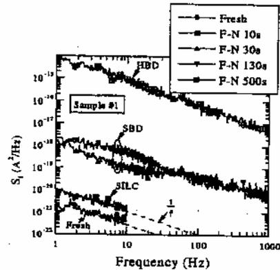
**Fig. 4:** Measured drain current noise spectra (SID) with  $V_{DS}=0,1V$  and  $V_{GS}=1V$  for several F-N stress times
