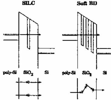
**Fig. 2:** Energy band diagram of the MOS structure with the trap assisted tunneling process for the SILC and the soft breakdown phenomenon.
