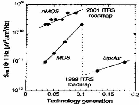
**Fig. 1:** ITRS roadmap for the  $1/f$  noise spectral density  $SV$  gate of a RF transistor. Note that  $SV$  gate is normalized to an active device area of  $1 \mu\text{m}^2$  and that  $SV$  gate  $\sim (W.L)^{-1}$ . The 1999 roadmap assumes a bipolar device through 110 nm and a MOS device for later generations. The effective gate bias, however, is not mentioned.
