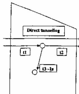
**Fig. 3:** Noise generation mechanism for trap-assisted tunneling current. Time  $t_3$  is slow relaxation for the trap that gives rise to fluctuations in the tunneling times  $t_1$ - $t_2$ . The time  $t_3$  is much larger than the tunneling times  $t_1$  and  $t_2$
