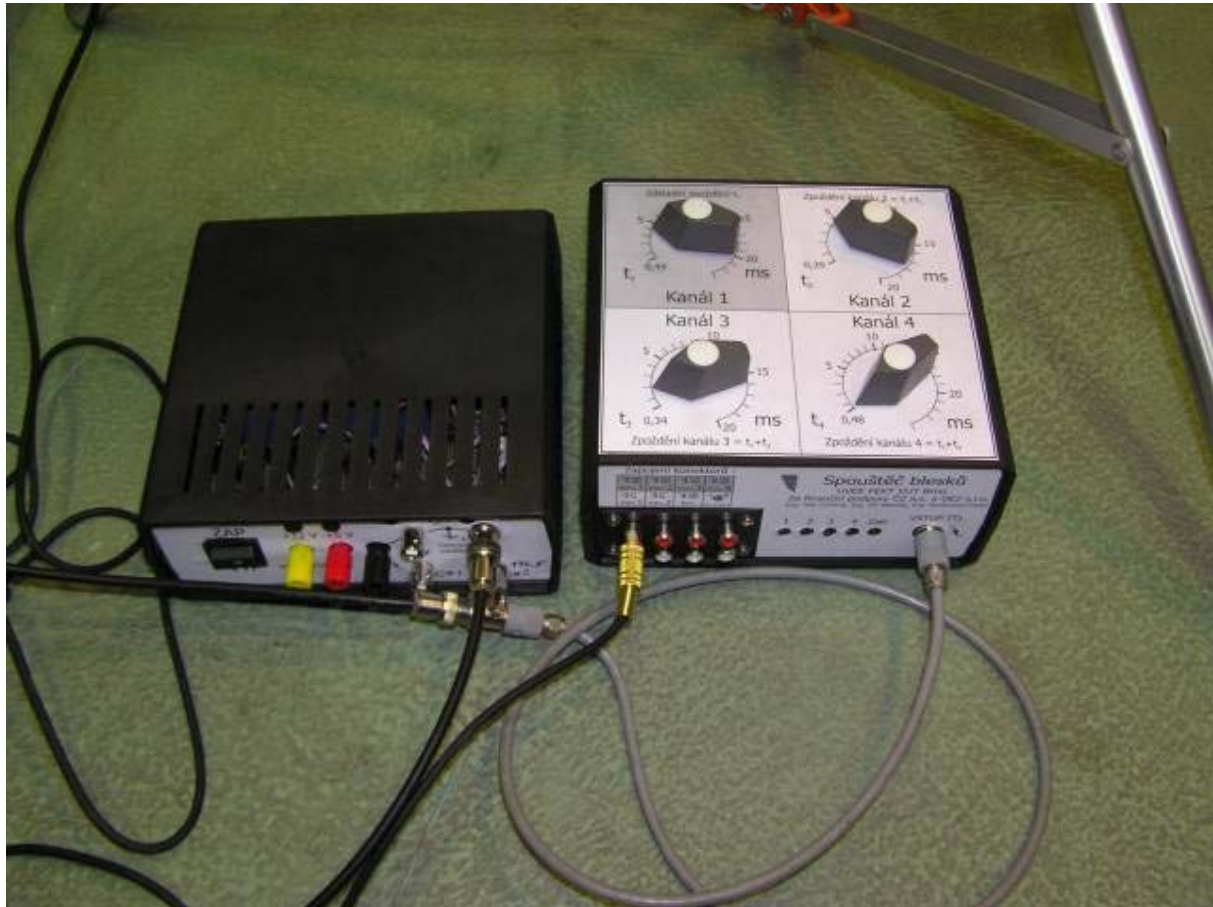
Fig. 4: Practical usage of signal convertor and timing device – gun shooting
