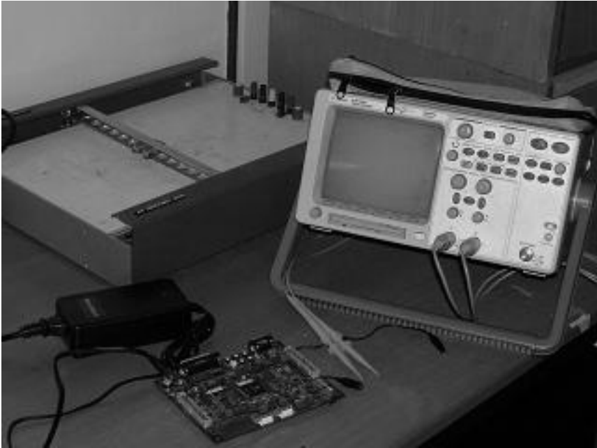
Fig. 3: Evolution dsp board with 2d plotting system and scope
