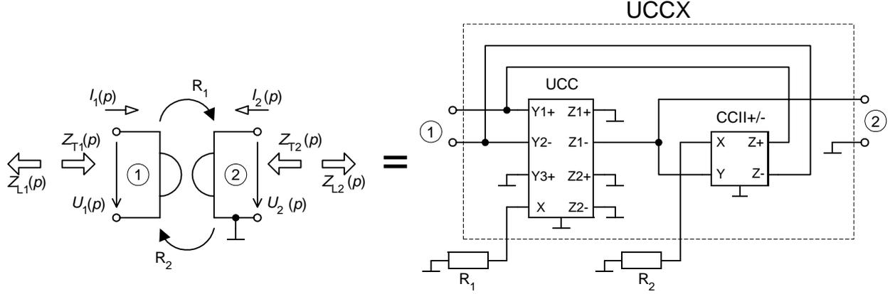
**Fig. 3:** Current conveyor UCCX acting as positive gyrator
