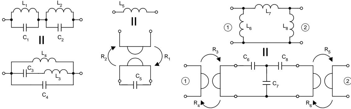
**Fig. 4:** Passive and active circuit transformations
