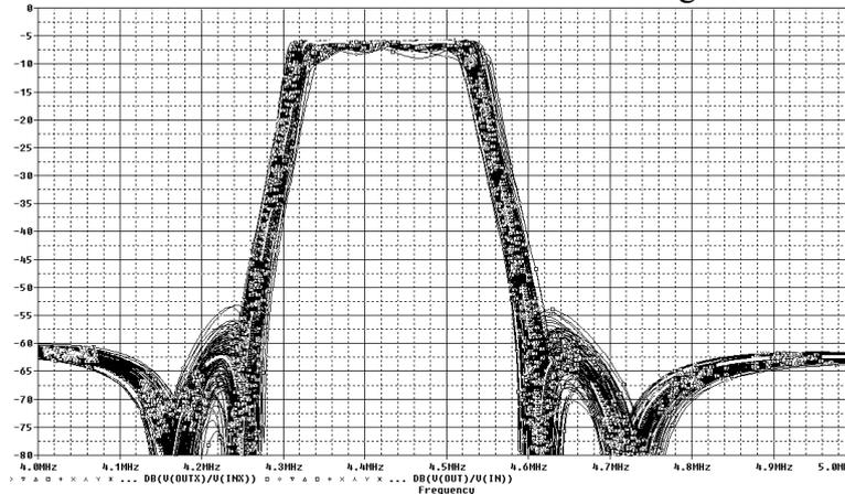
**Fig. 8:** Monte-Carlo analysis of band-pass magnitude response
