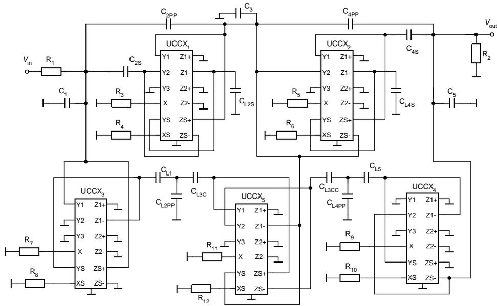
**Fig. 5:** ARC Cauer 5th order band-pass filter containing the UCCX devices
