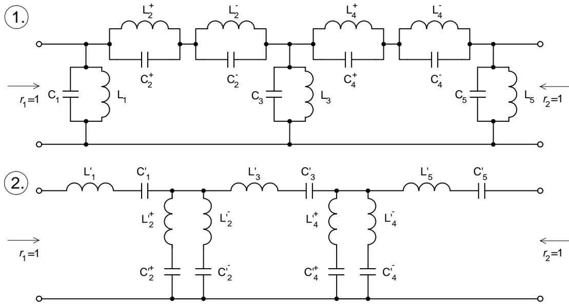
**Fig. 1:** Cauer RLC band-pass filters, 5<sup>th</sup> order
