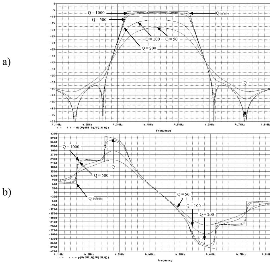
**Fig. 2:** Magnitude a) and phase b) frequency responses of the RLC band-pass filter
