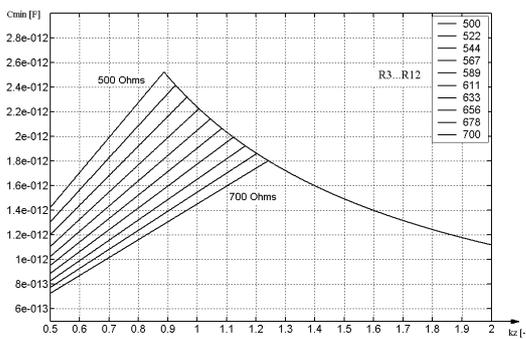
**Fig. 6:** Minimum capacity vs. impedance multiplication coefficient
