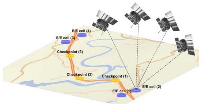
**Fig. 4:** Virtual Tolling System Architecture
