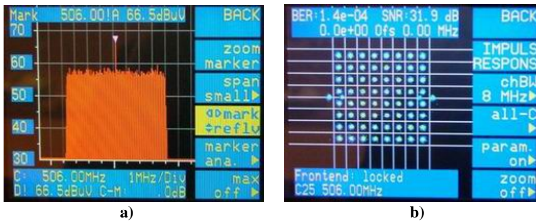
Fig. 2: MSK 33 receiver measurement: a) spectrum; b) constellation diagram
