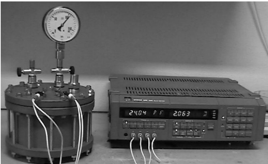
Fig. 1: The reaction chamber at estimation of the loss factor and relative permittivity
