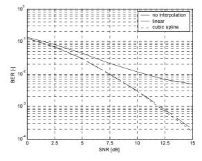
Uncoded BER performance for N = 50with none, linear and cubic spline interpolation
