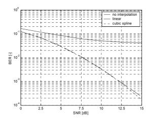
Fig. 3: Uncoded BER performance for N = 100with none, linear and cubic spline interpolation.
