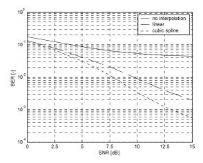
Fig. 4: Uncoded BER performance for N = 200 with none, linear and cubic spline interpolation
