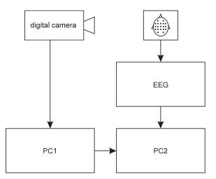
Figure 1: System for Synchronized EEG Recording and Sleep Movement Monitoring
