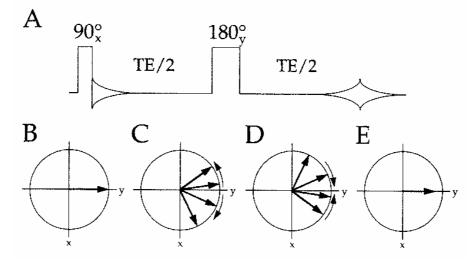
**Fig. 3:** Spin echo: a) pulse sequence, b-e) time-vector diagram (rotating frame – xy plane)
