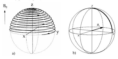
**Fig. 1:** Path of magnetization vector  $M_0$ : a) laboratory coordinate system, b) rotating coordinate system
