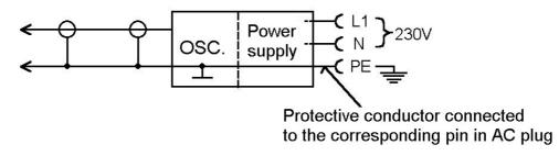
**Fig. 1:** Oscilloscope connection to the mains
