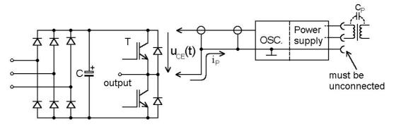
Fig. 2: Example of power electronics measurement
