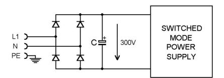
Fig. 3: Input side of an oscilloscope
