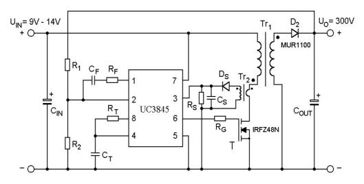
**Fig. 4:** *Wiring diagram of a converter*
