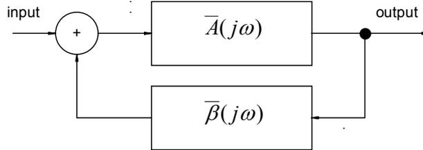
**Fig. 1:** *Linear feedback system as oscillator*
