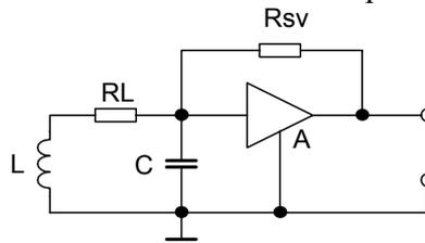
**Fig. 2:** *Simplified oscillator diagram*
