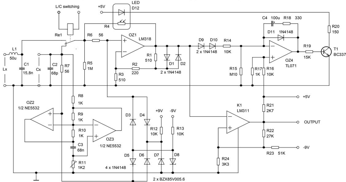
**Fig. 3:** *Measuring oscillator - circuit diagram*
